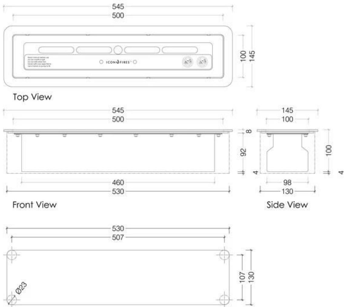
Slimline 500 Biofuel Burner With Mount Plate
