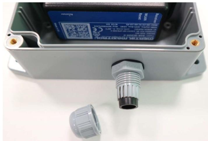
Place Wi-Fi Box cable through the nut (first) and sealed cable bushing into the protective box. Make sure that the rubber gasket stays on place
