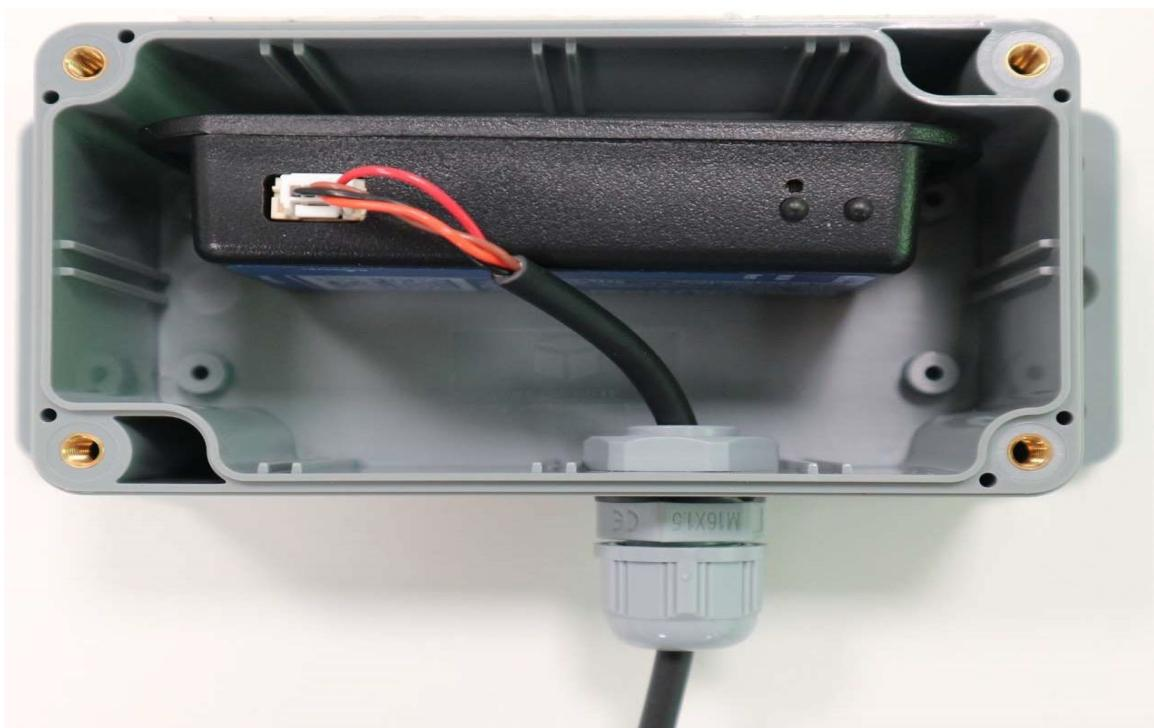
Place sealing gasket on the protective box cover
