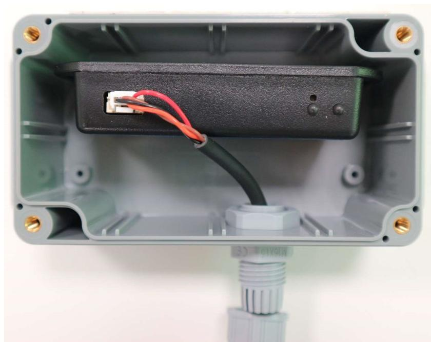
Screw the nut to seal the connection
