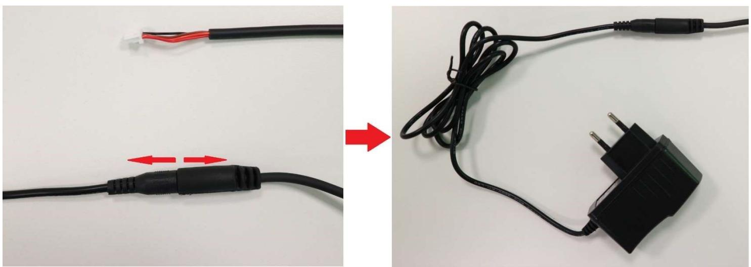
Unscrew the nut of cable bushing. Make sure that the rubber gasket is on place
