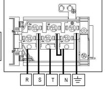
When you have finished to connect the equipments for the oven's power supply protection, make a functioning test using the instrument for testing the differential switch's efficiency.
