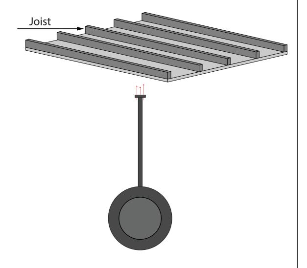
Attach the fireplace to the ceiling, using 3 appropriate screws and plugs, which are compatible with your celing.
