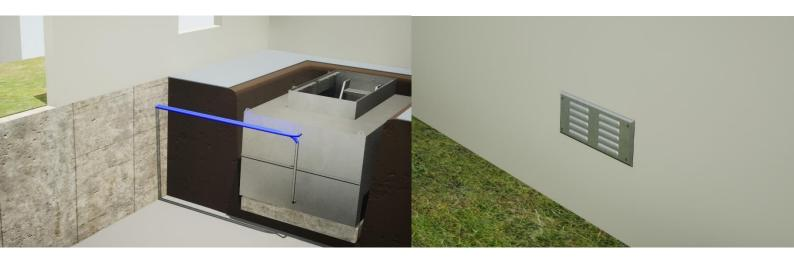
The ventilation hoses are connected to the dedicated openings in the wine cellar and led all the way out to an exterior wall. Here they are attached and hidden behind the ventilation grill that comes with the wine cellar. The purpose of the ventilation hoses is to ensure that the air in the wine cellar is constantly replaced. The wine cellar uses passive cooling and ventilation without the use of energy. Thus, it is neither a burden on the environment nor the electricity bill.
