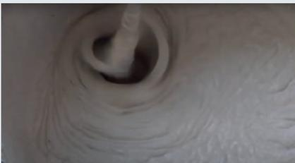
**1** Mix the plaster with water according to the stated mixing ratio.
